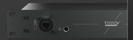
It connects to its dedicated ether CON connector, and can be used with any CAT6 network cable.
