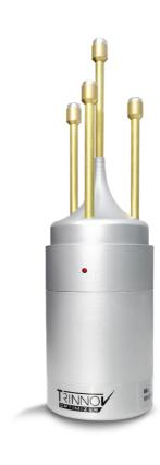
With many unique capabilities, the Optimizer's magic begins with Trinnov's iconic 3D Microphone. With 4 elements in a tetrahedral arrangement, this microphone captures sound in three dimensions, which the Optimizer uses to precisely locate the speakers, within 2° of azimuth and elevation, and 1 cm of distance. Exclusive to Trinnov, this microphone is factory calibrated to ±0.1 dB accuracy through an individual compensation file loaded onto the processor prior to the measurement.
